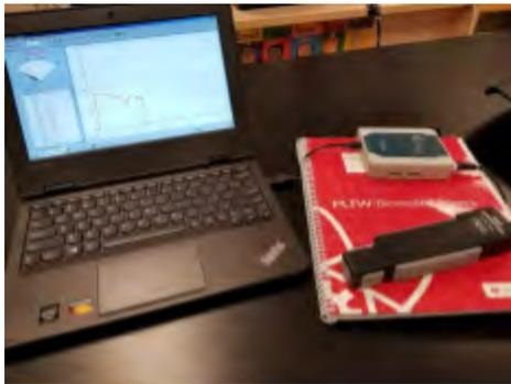
Student uses the LoggerPro program, their laboratory journal, and a hand dynamometer for their experiment.
